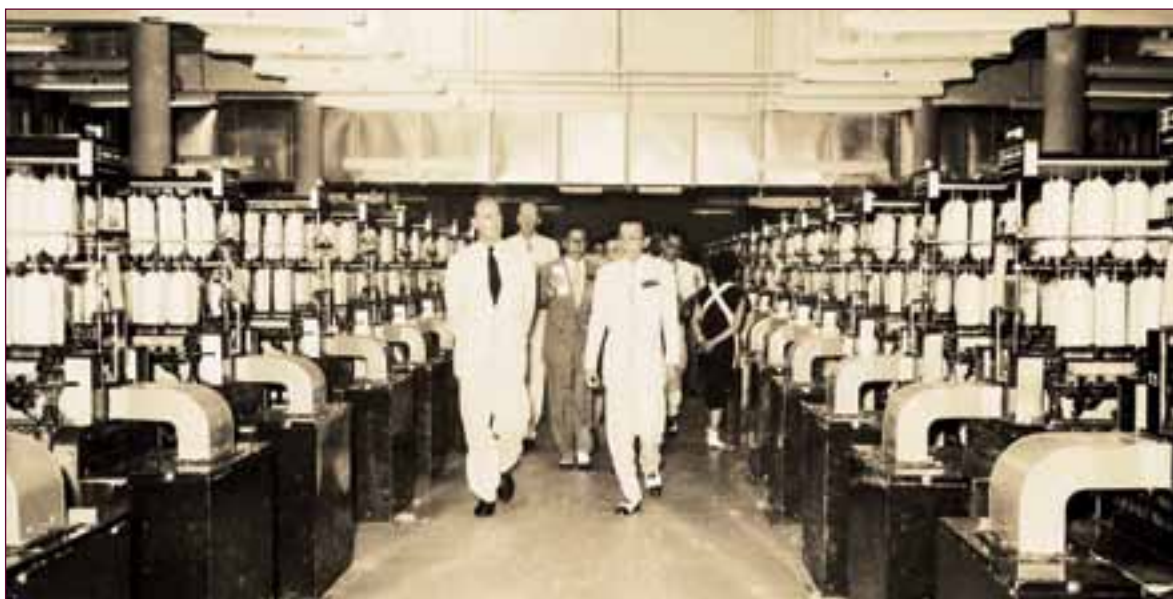
Sir Robert Brown Black, 23rd governor of Hong Kong (1958–1964), visits Hong Kong Spinners. Sir Robert and T.Y. Wong inspect the rows of ring spinning machines, all of which are equipped with a vacuum cleaning function.
