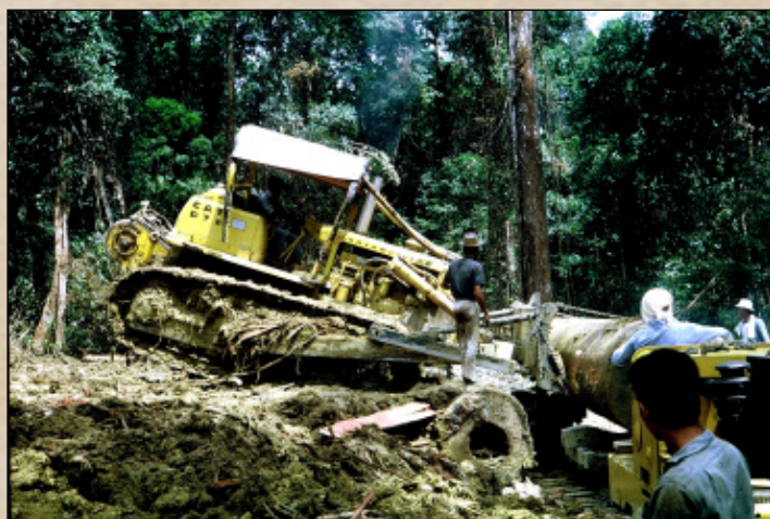
Plate 6: "Loading Log on Rail Dolly using Caterpillar D7E" North Borneo Timbers, Kretam. Photo K.V.Robinson circa 1968. Courtesy of Mrs. Judith Robinson.
